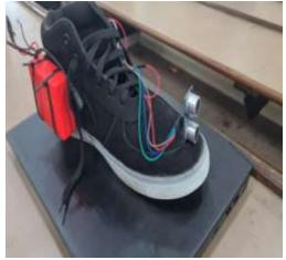
**Sensor integration**: Once the prototype is designed, the next step is to integrate the sensors into the shoes. This involves connecting the sensors to a microcontroller such as an Arduino board. The ultrasonic and IR sensors are typically connected to different digital pins on the Arduino board, and the voltage and ground pins are connected to the corresponding pins on the board.
