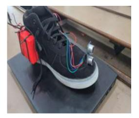
The ultrasonic and IR sensors in the shoes can detect obstacles and machinery in the user's path and provide real-time feedback through the display and alarm system, allowing the user to safely navigate through the workspace. Additionally, the shoes' compact and portable design makes them easy to useand wear in any environment.
